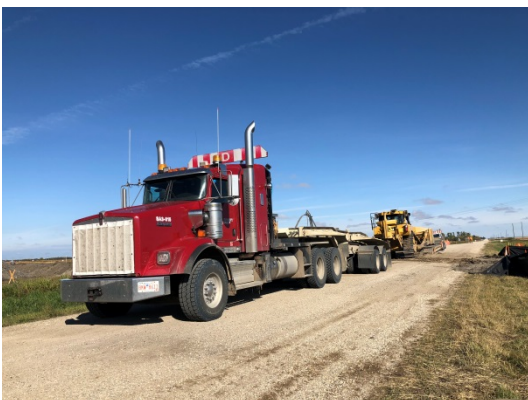
SF 47, photo facing north, lowbed came to pick up 4 dozers total and move them.
